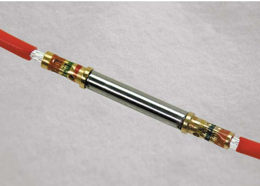
An example of a good crimp showing the exposed wire.
