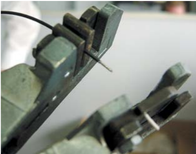
Wire stripping with a recommended tool will allow the insulation to be removed accurately without damaging the wires.
