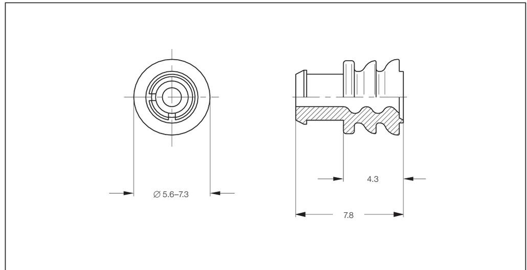
**Diameter 1.5 mm Pin and Socket Contact**
