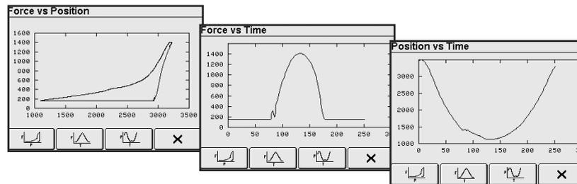
Detailed display of real time crimp data is readily available to the operator.
