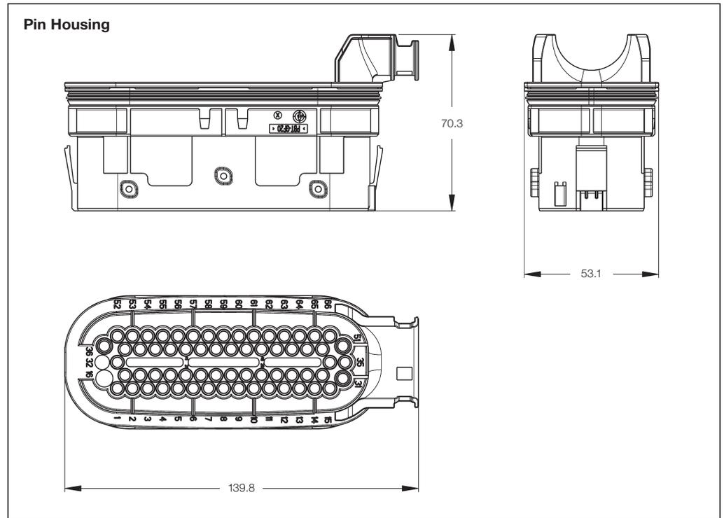
**Sealed Pin Housings with Secondary Locking Device**
