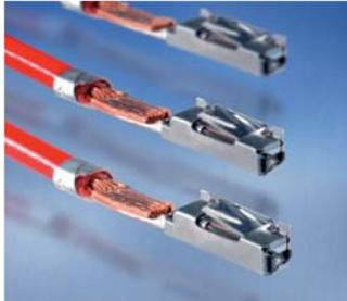
Tyco Electronics offers semi- and fully-automatic modules for resistance compact welding of terminals. This resistance welding process allows us to achieve minimum transitional resistance between conductor and contact, higher current capacity and long-term stability of the wire termination.
