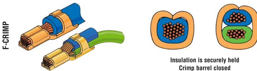
For double wire applications with different size wires always place wire with smallest outer diameter in the bottom
