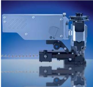
The System III Applicator revolutionizes the traditional applicator market by separating the feed and the termination. When the feeder is attached to the applicator, the system reads the specific terminal information from the onboard iButton™ data module permitting the automation of many manual adjustments such as crimp height, feed pitch, etc.
