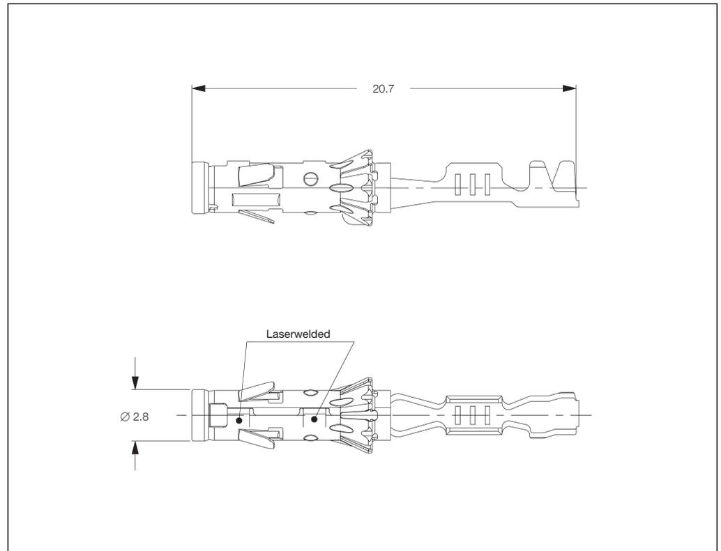
**Socket Contacts for Diesel Fuel Injector Connector**
