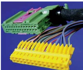
The development of this termination machine was necessary to be able to process high cavity-count female connectors in IDC technology. The new multi-cavity motor-control interface connectors are used in damp areas in cars and must be
