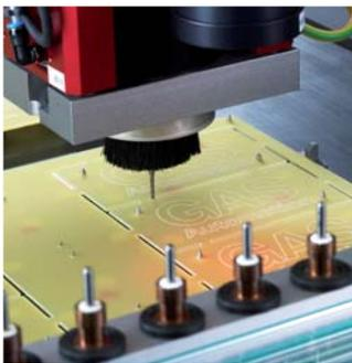
The GAS SAR-1000-B and SAR-1000-D depanelling systems for printed circuit boards and bare boards offers a largely automated process for depanelling by milling and/or sawing.
