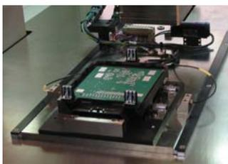
A key feature of the SEP press system is an automatic shuttle that positions the PCB and housing\connector stack up underneath the upper insertion tool.
