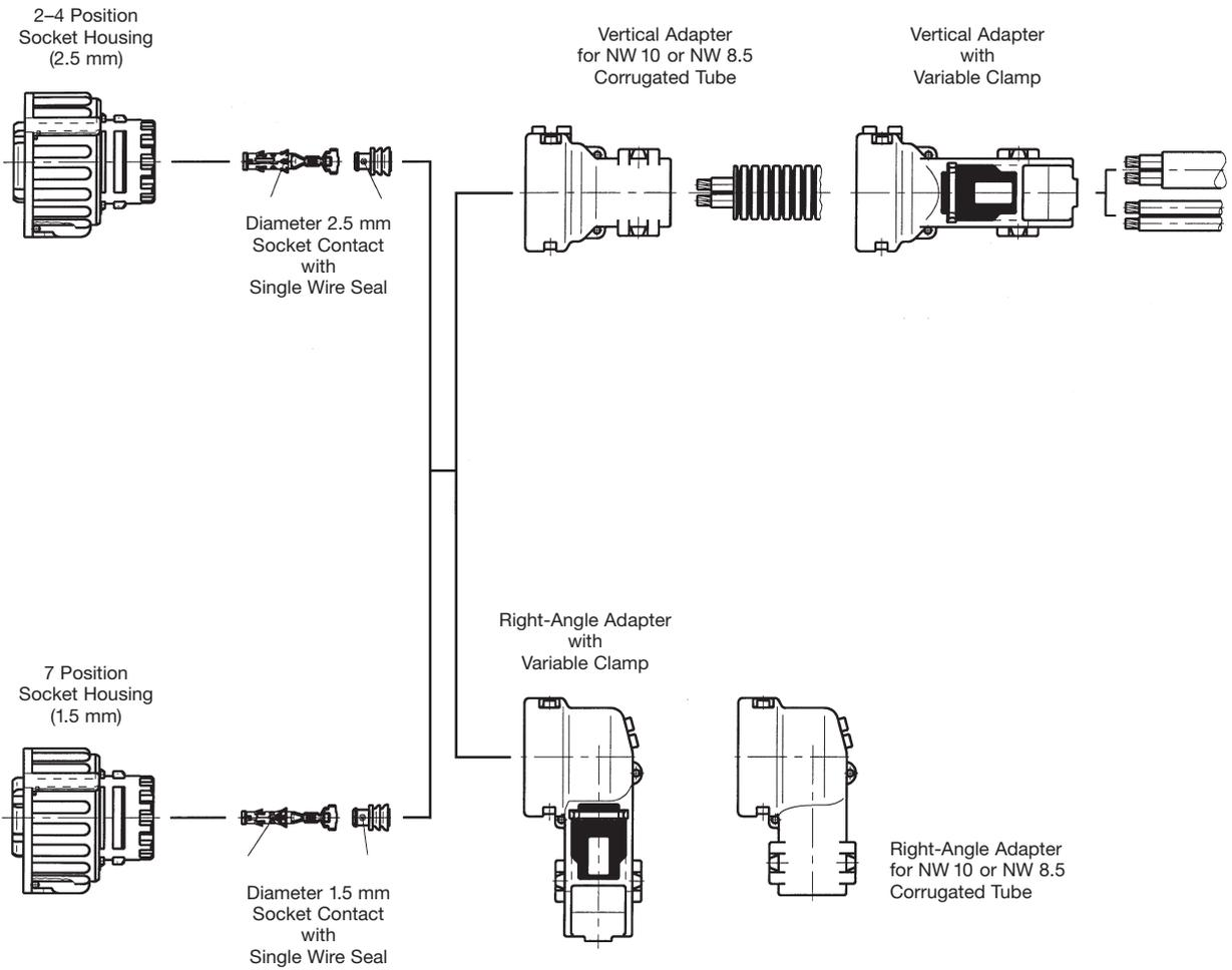
Sealed Pin Connector Assembly
